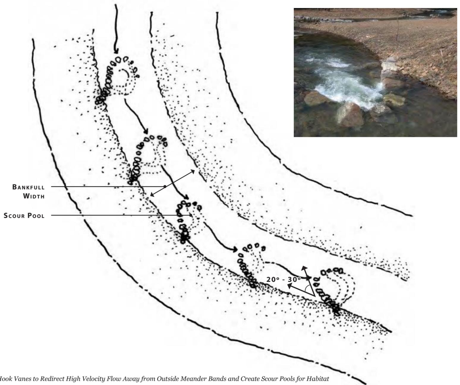
Figure 13. Use of J-Hook Vanes to Redirect High Velocity Flow Away from Outside Meander Bands and Create Scour Pools for Habitat
