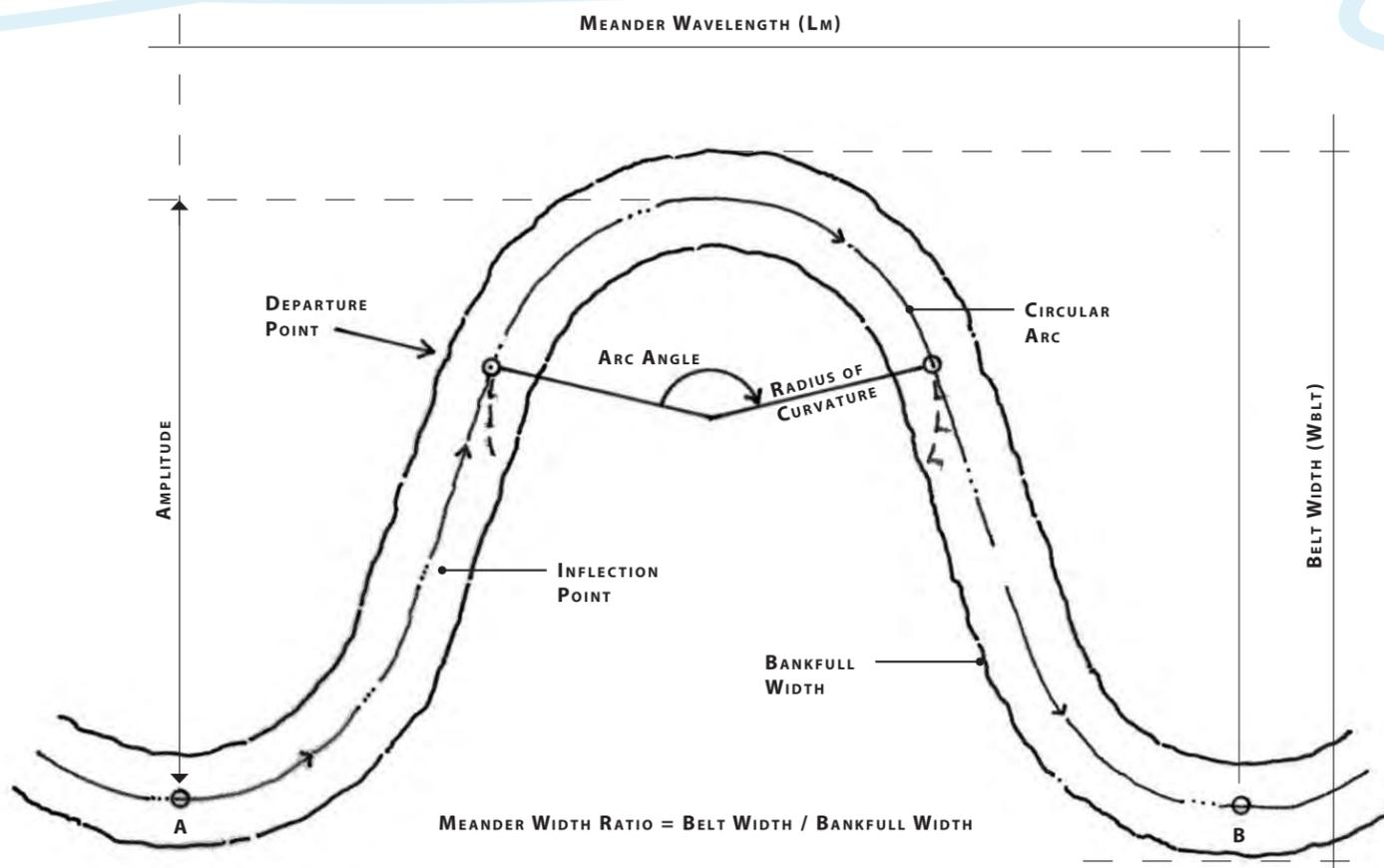
Figure 6. Plan View Characteristics (Rosgen, 1996)
