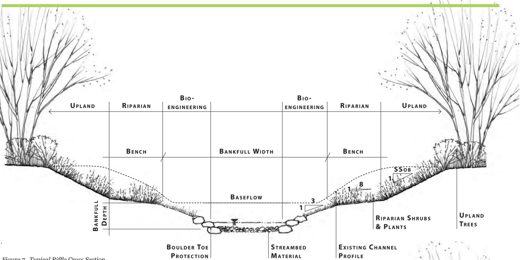
Figure 7. Typical Riffle Cross Section
