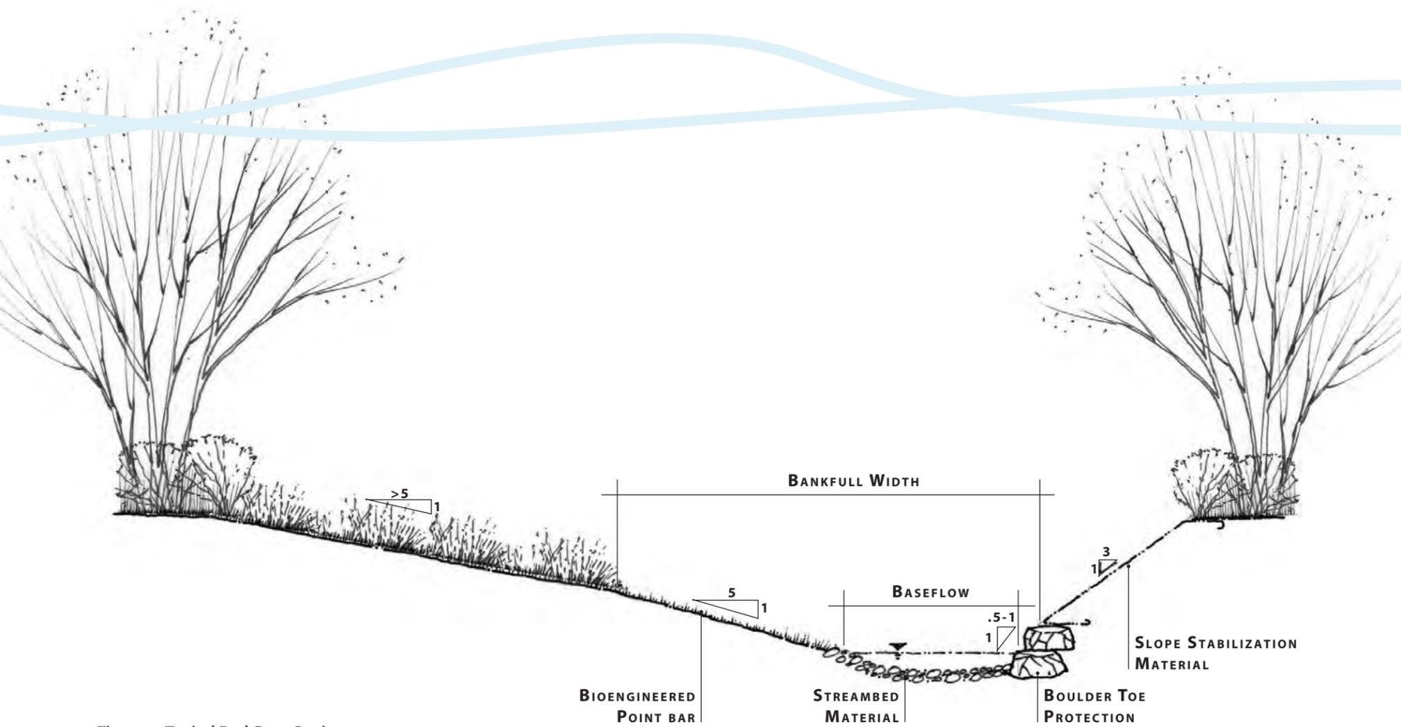
Figure 9. Typical Pool Cross Section
