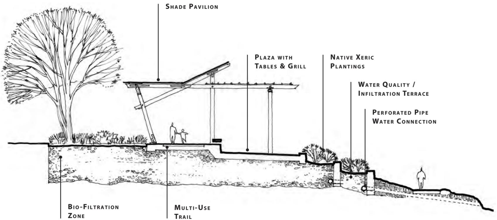
Figure 20. Bio-Filtration allows for natural processes to clean runoff before entering the streams.
