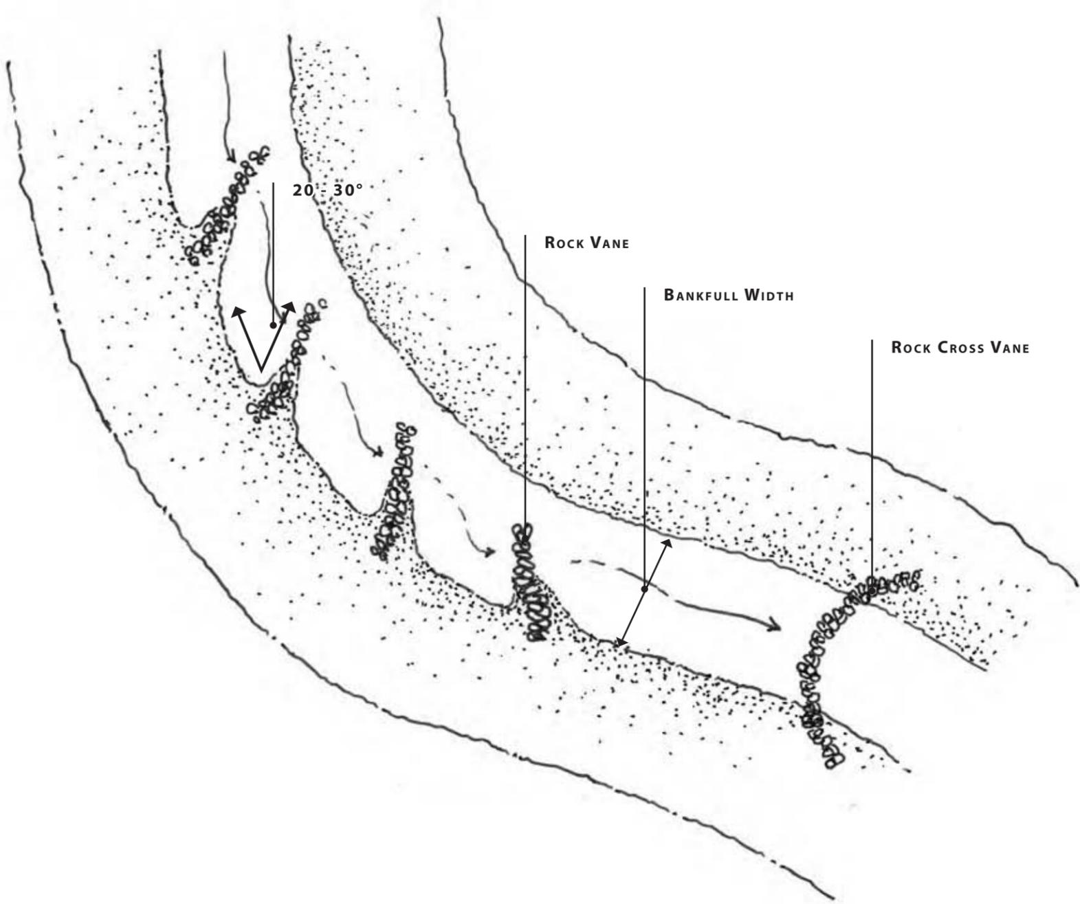
Figure 10. Use of Rock Vanes to Protect Outside Meander Bends
