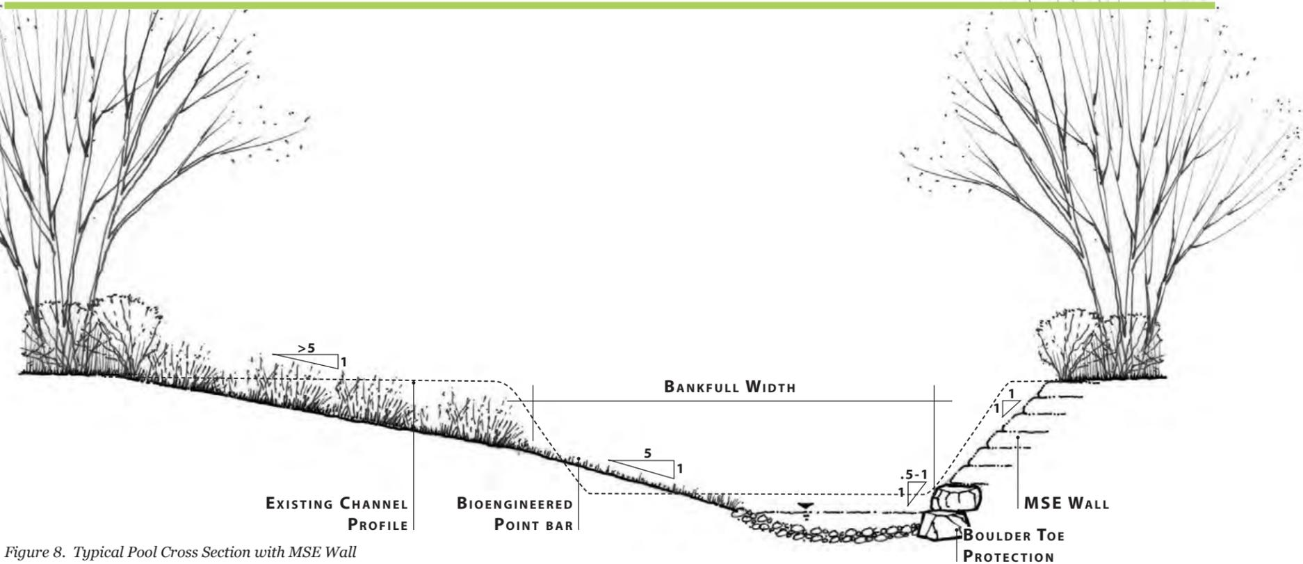
Figure 8. Typical Pool Cross Section with MSE Wall
