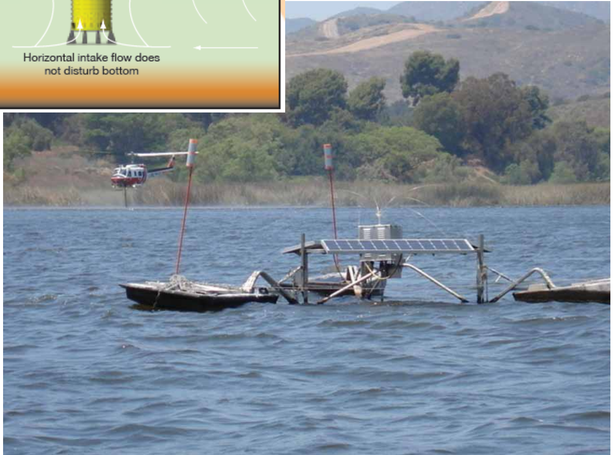
Figure 5.5: Diagram and Image of SolarBee Mixer
