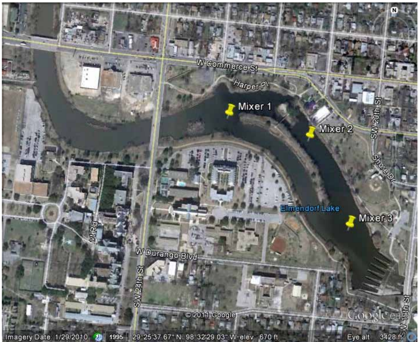
Figure 5.6: Proposed Locations of SolarBee Mixers (Source of satellite image: Google Earth)
